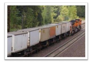
However, since the 1970s, the concept of piggybacking has given the railroads a boost. This is where loaded highway trailers are loaded onto railcars, and taken to railheads. From there, local trucks take the trailers the rest of the way to their destination.
