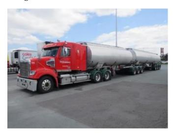
**B-Train:** Consists of two trailers connected by a fifth wheel.
